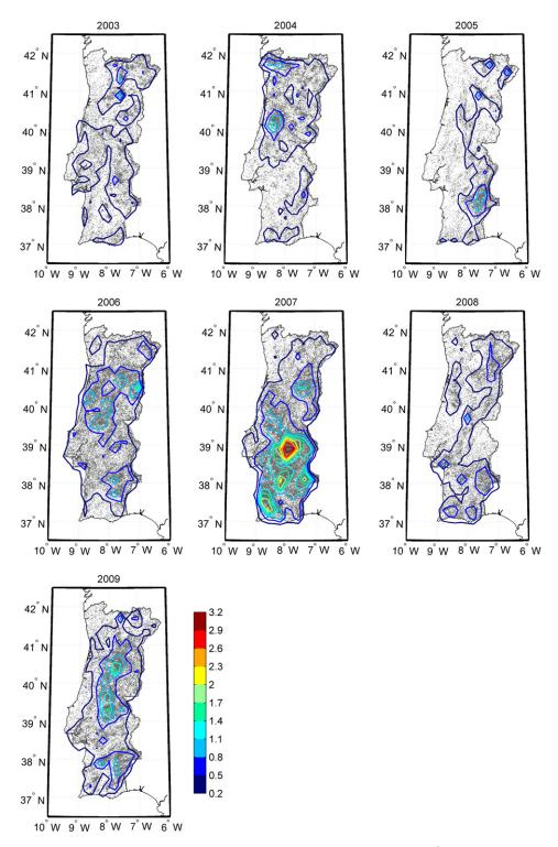
**Fig. 2.** Spatial density distribution of CG discharges in coloured contours. Values given as number of discharges/km<sup>2</sup> per year over a regular 0.2°×0.2° grid. All effective CG discharges for each year are represented by grey dots.
