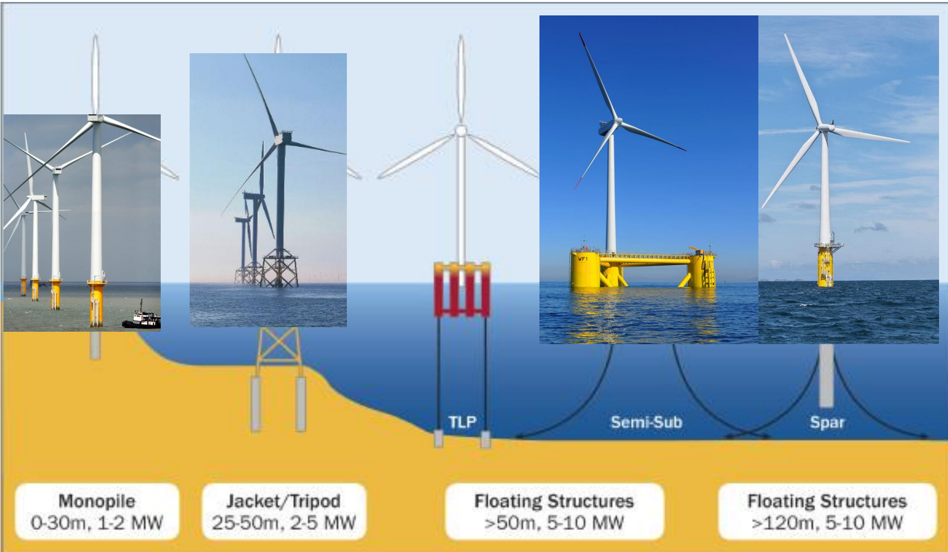
Fig. 6: Offshore wind concepts (Source: researchgate.net; power-technology.com; iearth.org; pagerpower.com)
