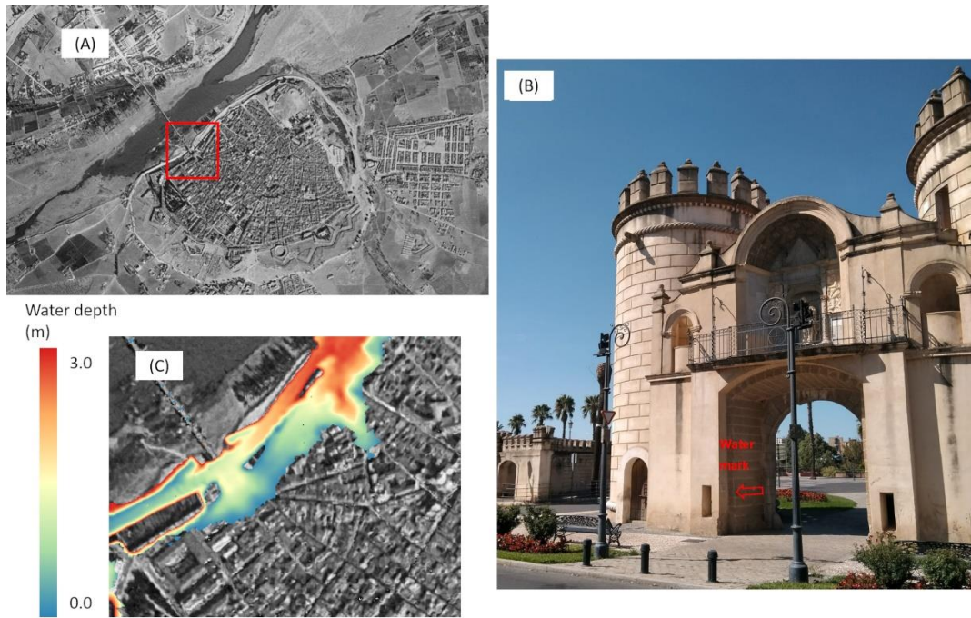
Figure 11. Maximum water depth obtained in the Palmas Gate. Panel (A): location of the control zone (area inside the red box); Panel (B): water mark in the Palmas Gate; Panel (C): numerical results of maximum water depth.
