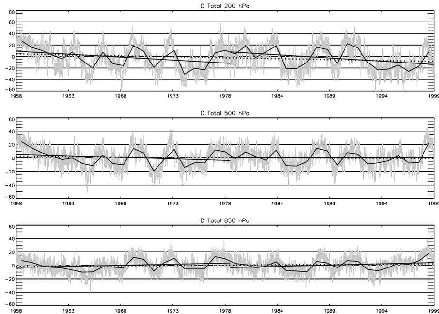
**Fig. 2.** Daily evolution of indices  $D_{\text{GLOBAL}}$  at 200 hPa, 500 hPa and 850 hPa. 365 days moving average and trend line are overplotted in the three figures. (X-axis: time, Y-axis: percentage of the area covered by high temperature that exceed that covered with low temperature). Trends for the subperiods 1958–78 and 1979–98 are included.
