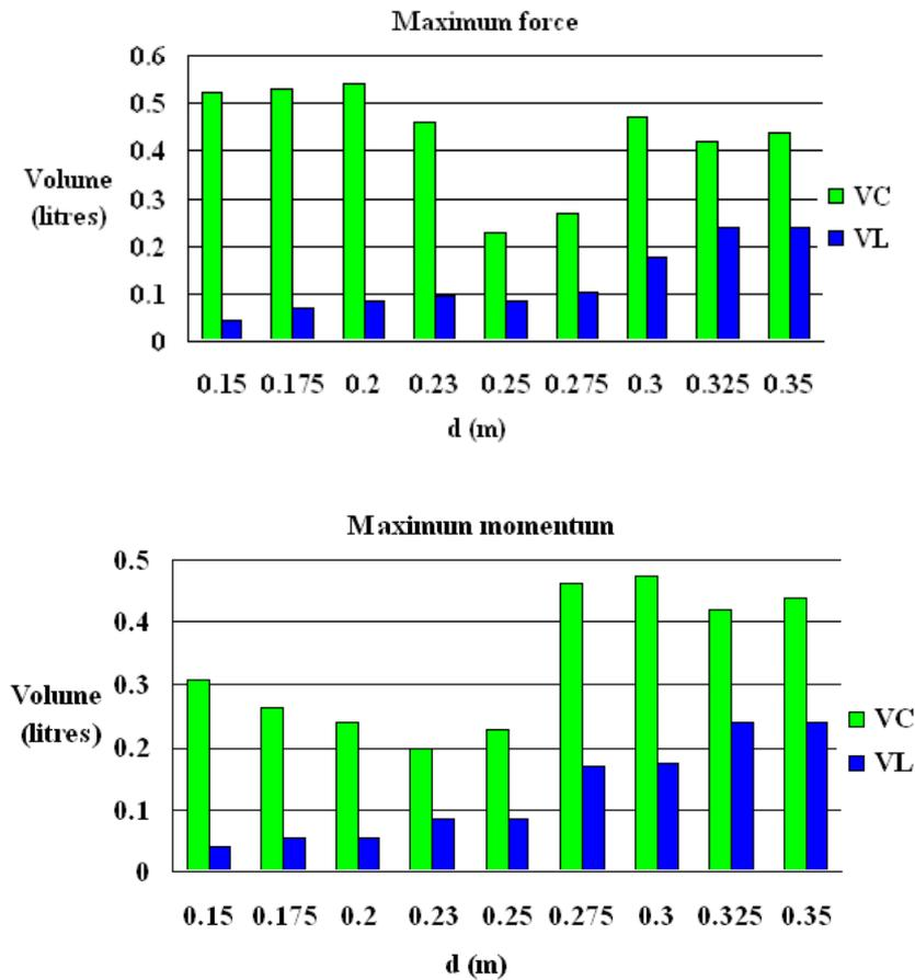
Figure 6.14: Volume of water classified according to their origin at the instants of maximum force and moment ( $H_D = 0.05m$ ).  $V_C$  corresponds to the water initially placed at the central band ( $Y \in [0.24, 0.36]$ , see Figure 6.5).  $V_L$  corresponds to the water initially placed at the lateral bands.
