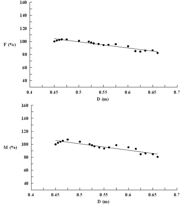
Figure 6.6: Dependence of the force and moment calculated without protection barrier on the distance between the dam break and the structure.
