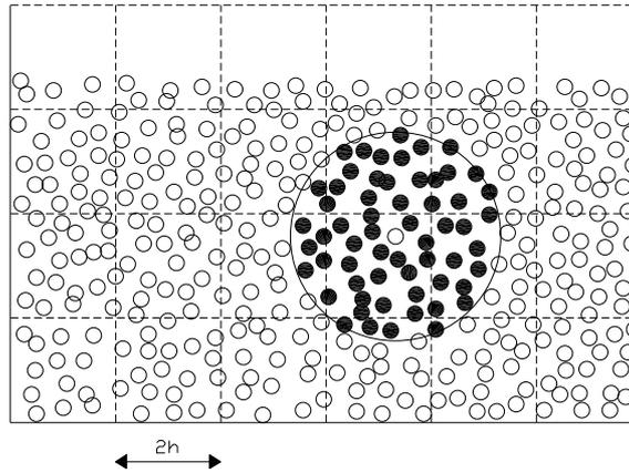
Figure 3.8: Set of neighboring particles in 2D. The possible neighbors of a fluid particle are in the adjacent cells but it only interacts with particles marked by black dots.
