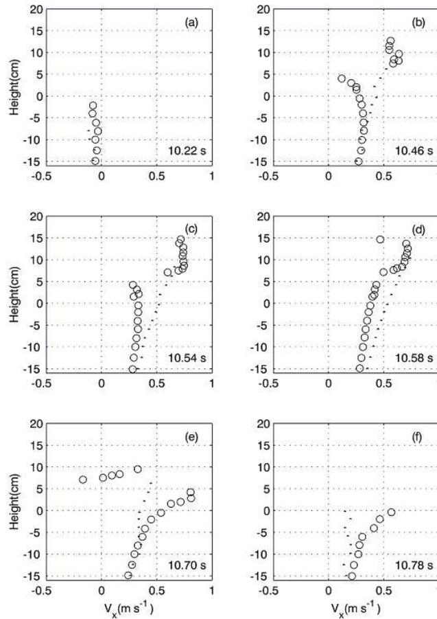
Figure 4.6: Vertical variation of experimental horizontal velocity. Data without deck ( $\bullet$ ) and with deck ( $\circ$ ). Velocities were measured at the leading edge of the deck ( $x = 8.0m$ ).
