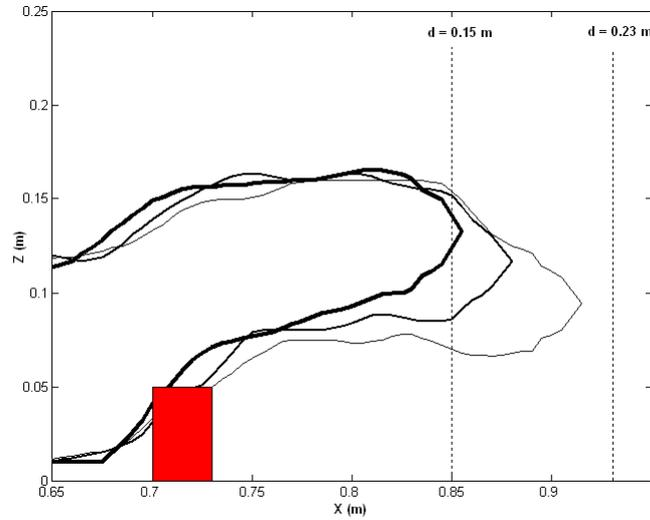
Figure 6.11: Jet profile corresponding to different instants during dike overtopping. The vertical lines correspond to the region with a sharp decrease in moment ( $H_D = 0.05m$ ).
