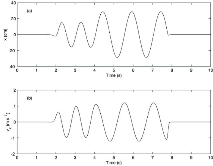
Figure 4.4: Wavemaker signal for transient wave generation. (a) Horizontal displacement; (b) Horizontal velocity.
