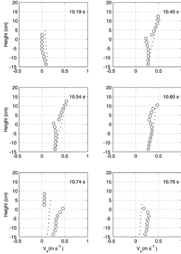
Figure 4.7: Vertical variation of numerical horizontal velocity. Data without deck (●) and with deck (○). Velocities were measured at the leading edge of the deck ( $x = 8.0\text{m}$ ).
