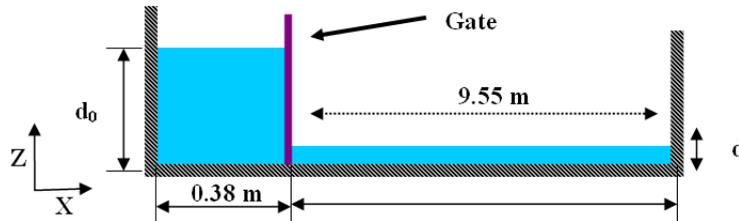
Figure 5.3: Schematic arrangement of the dam-break experiments.
