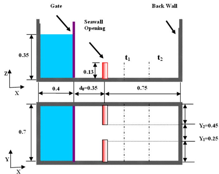
Figure 6.24: Configuration of the experiment corresponding to wave collision with an open wall.
