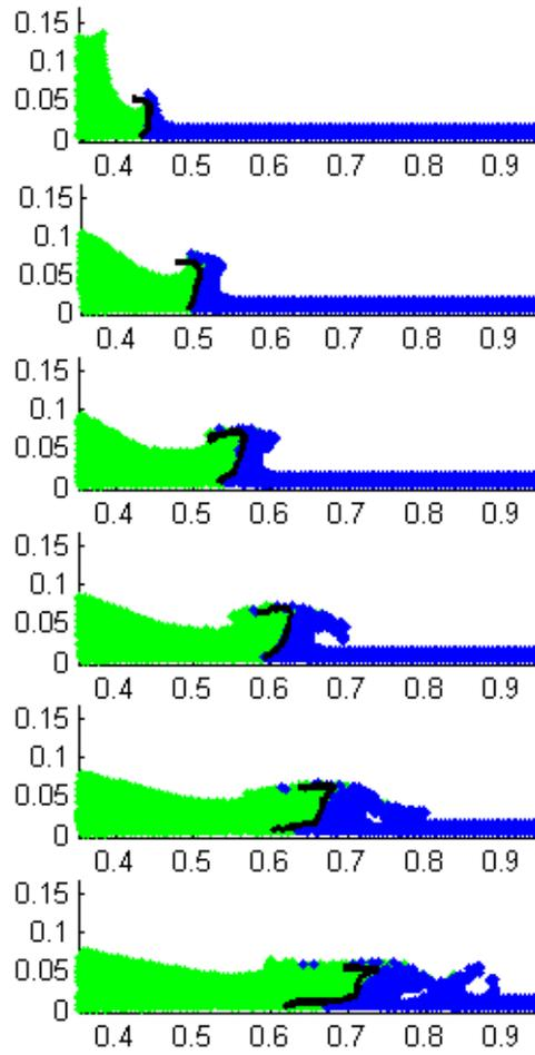
Figure 5.8: Experimental and numerical interface between lock and tank water ( $d = 0.015m$ ). Green color corresponds to lock water, blue color to tank water and the black line to the experimental interface.
