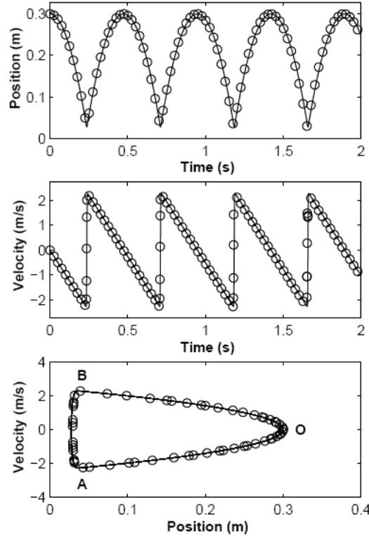
Figure 3.15: Single particle collision with a boundary in the absence of viscosity ( $\alpha = 0$ ).
