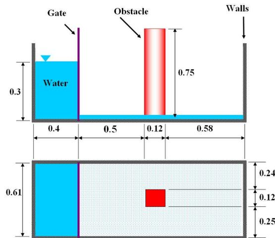
Figure 6.2: Initial configuration of the numerical experiment corresponding to interaction wave-structure.
