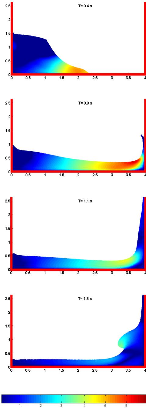
Figure 3.21: Collapse of a water column in a tank simulated with SPH model plotting the particle velocities.
