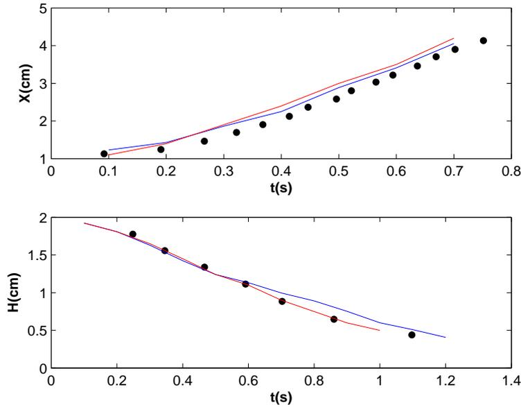
Figure 3.22: Collapse of a water column in a tank simulated with SPH model (blue solid line) comparing with experimental data (circles) and [Violeau and Issa, 2006] results (red solid line).
