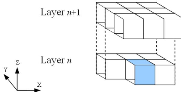
Figure 3.10: Sweeping through grid cells in 3D. Only 13 out of 26 possible neighboring cells are considered when centered on a particular  $ijk$  cell. The rest were previously considered when centered on adjacent cells using reverse interactions.
