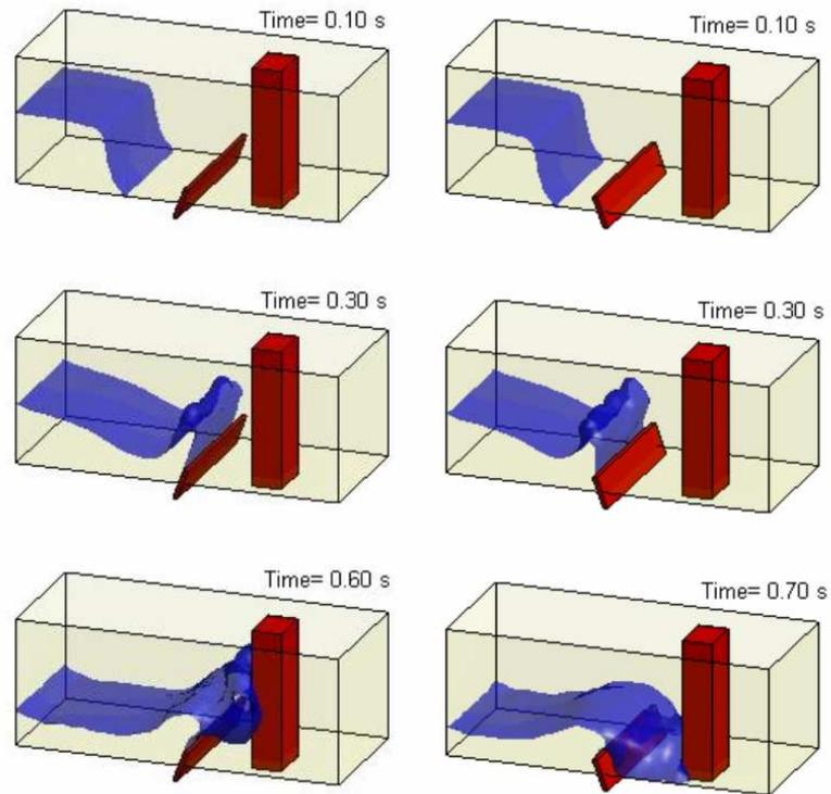
Figure 6.21: Different instants of the wave collision with a structure using a wall sloped landward (left) or seaward (right).
