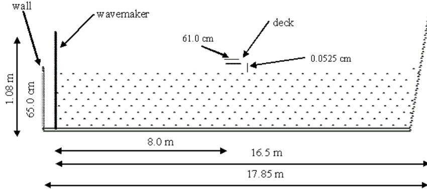
Figure 4.3: Initial SPH configuration of fluid and boundary particles to mimic the experimental setup shown in Fig. 4.2.
