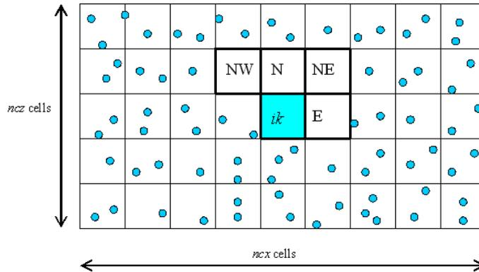
Figure 3.9: Sweeping through grid cells in 2D. Starting from the lower left corner, particles inside the center cell  $ik$  interact with adjacent cells only in E, N, NW and NE directions. The interactions with the rest of the cells W, S, SW SE directions were previously computed using reverse interactions.
