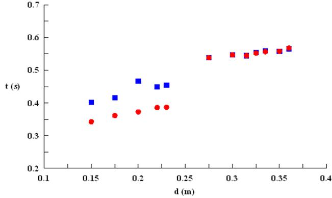
Figure 6.13: Dependence of the instants of maximum force and moment on the distance from the dike to the structure. The instants of maximum force (blue squares) are delayed with respect to the instants of maximum moment (red circles) for short distances.
