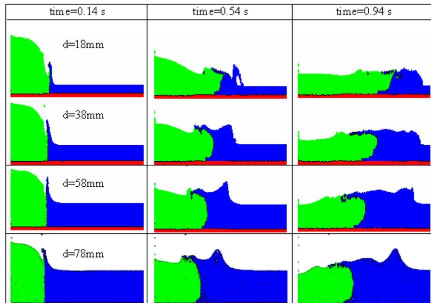
Figure 5.9: Different instants of dam evolution for different fluid depths. Green color corresponds to lock water and blue color to tank water.
