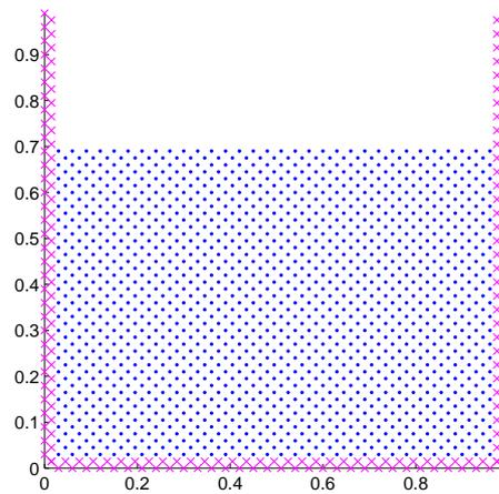
Figure 3.12: Sketch of the initial positions for a staggered grid. Crosses represent boundary particles and points represent fluid particles.
