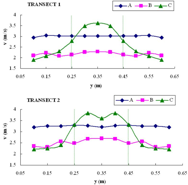
Figure 6.26: Measured velocity along the lateral extent. A: without wall. B: continuous wall. C: open wall.
