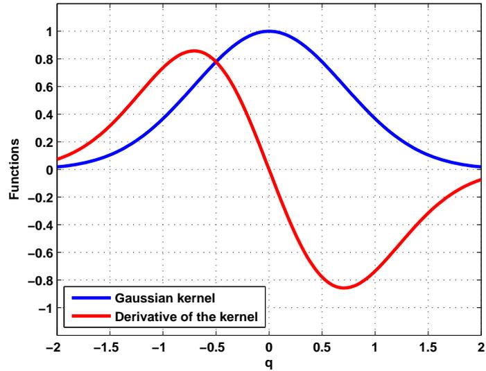
Figure 3.1: Gaussian kernel and its derivative divided by the dimensional factor  $\alpha_D$
