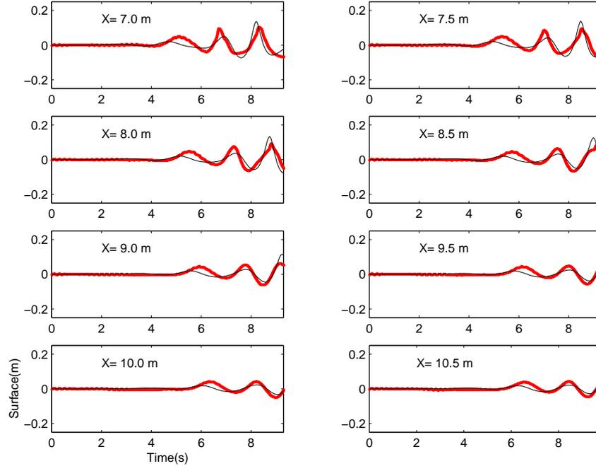
Figure 4.5: Free surface measurements in absence of deck. Comparison between numerical signal (heavy solid line) and experimental signal (light solid line).
