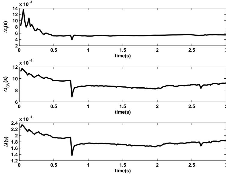
Figure 3.7: Time-step control in the collapse of a water column.
