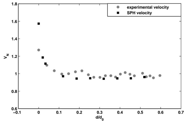
Figure 5.6: Comparison between experimental (light circles) and numerical (dark squares) dam-break velocity. The velocity was averaged in space during the first 3m in both cases.
