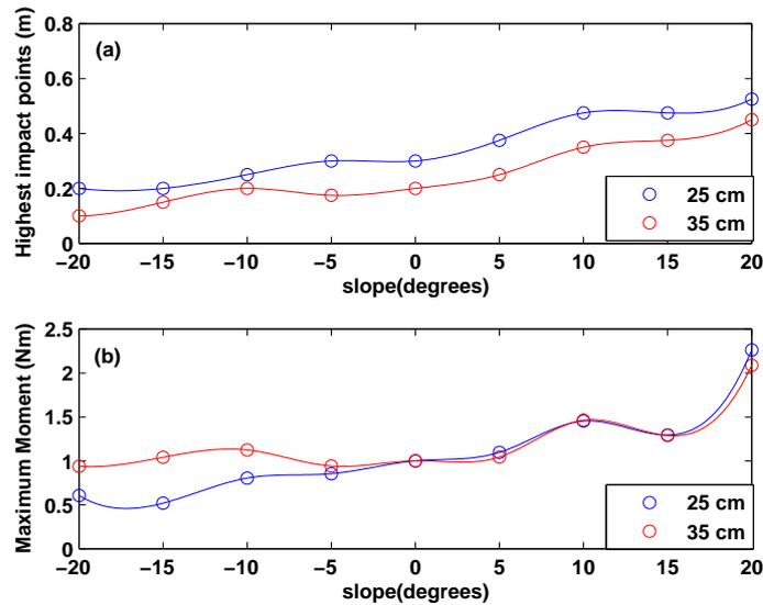
Figure 6.22: Dependence of highest impact points (a) and moment (b) with different wall slopes.
