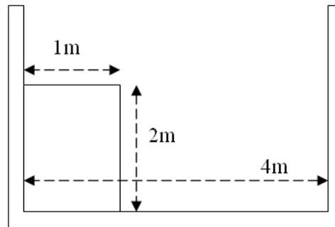
Figure 3.20: Initial configuration of the water column and the tank experiment.
