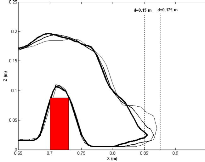
Figure 6.16: Water profile corresponding to different instants during dike overtopping. The vertical lines correspond to the region with a sharp increase in moment ( $H_D = 0.0875m$ ).
