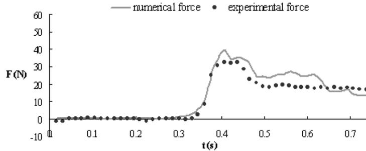
Figure 6.3: Comparison between numerical (solid line) and experimental (dark circles) forces exerted by the incoming wave on the structure.
