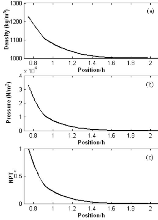
Figure 3.14: Variation of density (a), pressure (b) and normalized pressure term (c) for a moving particle approaching a solid boundary. Calculations were run without viscosity.
