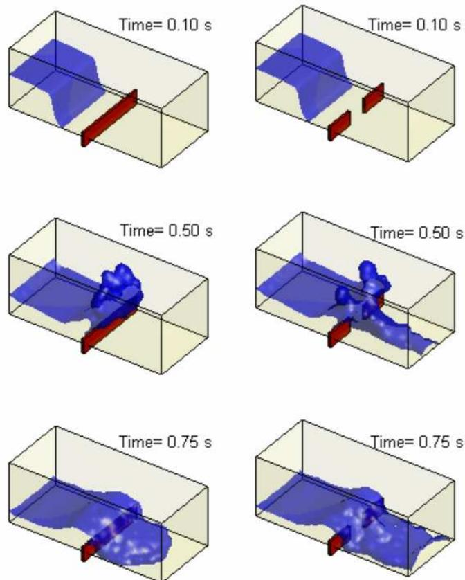
Figure 6.25: Different instants of the wave collision with a continuous wall (left frames) an open wall (right frames).
