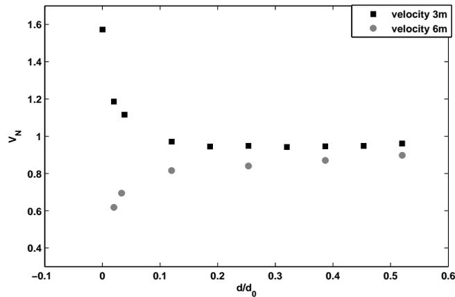
Figure 5.10: Spatial average of the velocity along the first 3 meters (dark squares) and the first 6 meters (light circles) for different fluid depths ( $d$ ).
