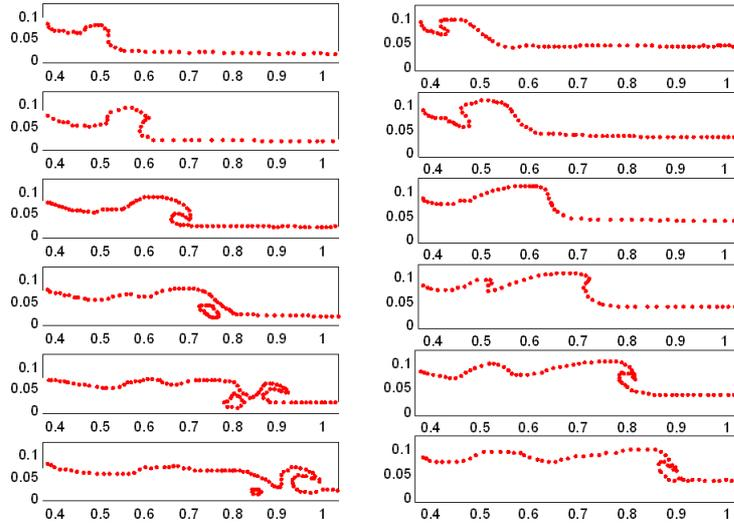
Figure 5.2: Experimental profiles digitized from Figure 2 in the paper of [Janosi et al., 2004]. The fluid depth in front of the lock is  $d = 18\text{mm}$  in the left frames and  $d = 38\text{mm}$  in the right ones.
