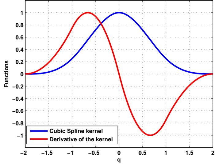
Figure 3.3: Cubic Spline kernel and its derivative divided by the dimensional factor  $\alpha_D$
