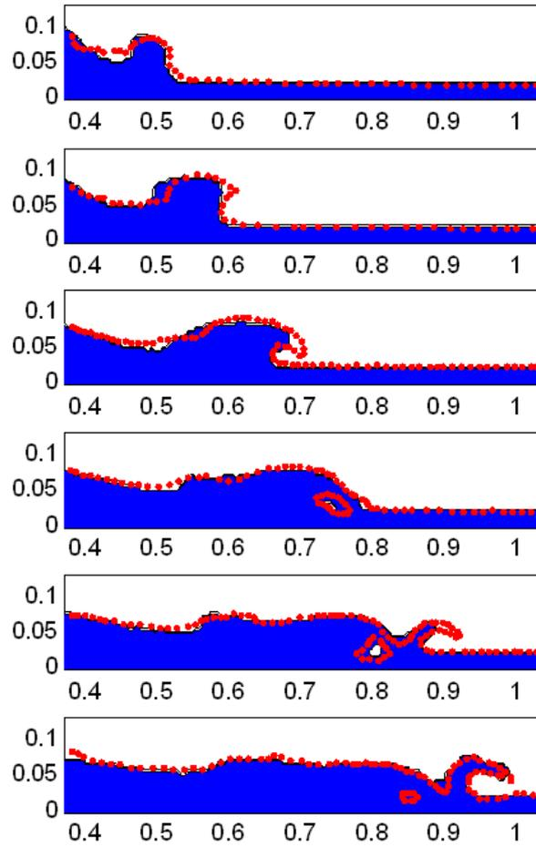
Figure 5.4: Comparison between experimental and numerical profiles of dam-break evolution over a wet bed ( $d = 0.018m$ ). Experimental values are represented by red dots and numerical ones by the blue surface.
