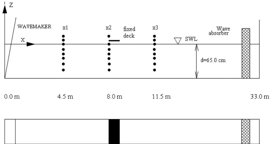
Figure 4.2: Elevation and plan view of experimental setup of Cox and Ortega.
