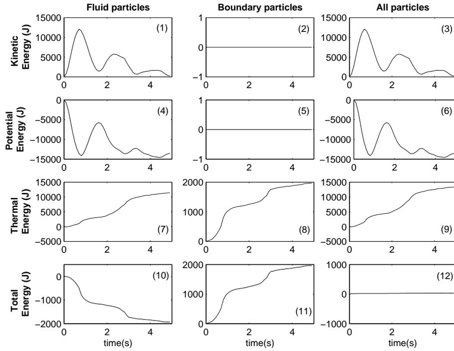
Figure 2.2: Time variation of the system energy during dam-break evolution.
