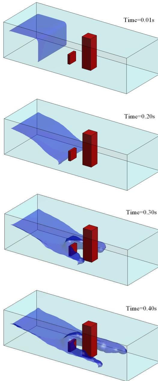
Figure 6.8: Different instants of wave-structure impact mitigated by a tall dike.
