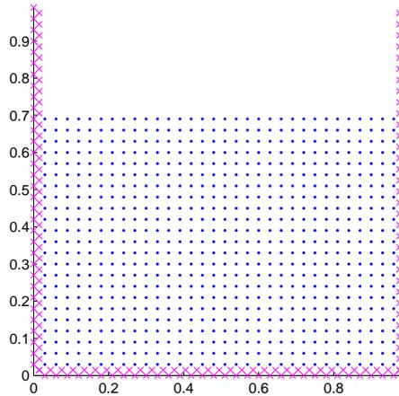
Figure 3.11: Sketch of the initial positions for a Cartesian grid. Crosses represent boundary particles and points represent fluid particles.
