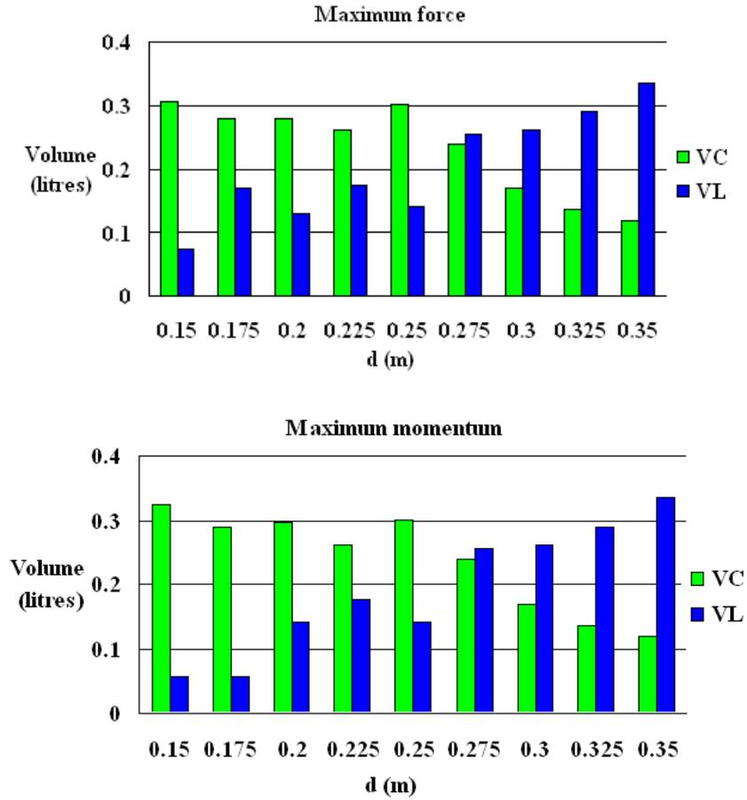
Figure 6.17: Volume of water classified according to their origin at the instants of maximum force and moment ( $H_D = 0.0875m$ ).
