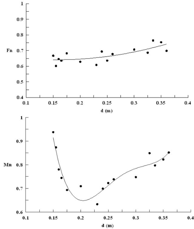
Figure 6.9: Dependence of the normalized force ( $F_n$ ) and normalized moment ( $M_n$ ) on the distance dike-structure for a tall dike ( $H_D = 0.05m$ ).
