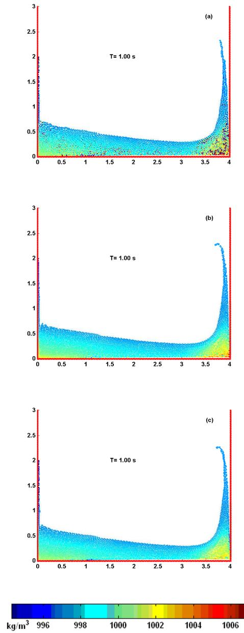
Figure 3.6: Density field for simple 2-D Dam break showing effect of density filters. (a) corresponds to AV, (b) corresponds to AV with Shepard filter and (c) corresponds to AV with MLS filter.
