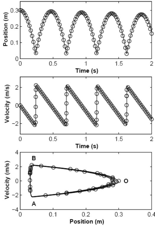
Figure 3.17: Single particle collision with a boundary in a viscous medium ( $\alpha = 0.05$ ).
