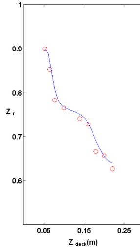
Figure 4.10: Relative height of the jet ( $Z_r$ ) decrease in terms of the distance between the free surface at rest and the deck. The same piston displacement,  $A = 0.25$  m and  $t = 2s$ , was considered in all simulations.
