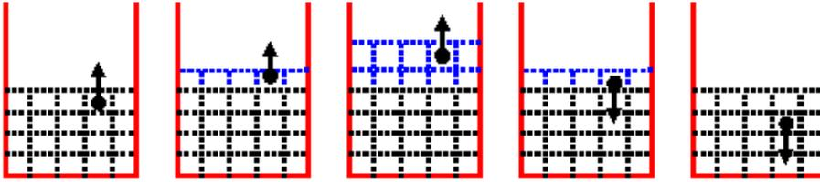
Figure 3.23: Evolution of new cells in  $Z$  direction depending on the fluid particles movement.
