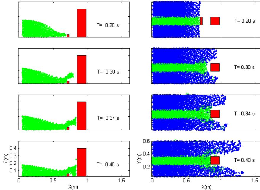
Figure 6.12: Lateral and top view of the water collision with the dike and the structure ( $H_D = 0.05$  m and  $d = 0.15$  m).
