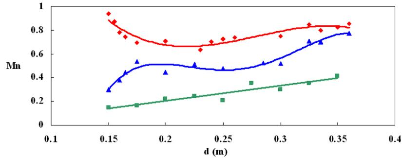
Figure 6.19: Dependence of the normalized moment ( $M_n$ ) for different distances dike-structure and different dike heights normalized  $H_D$ ;  $H_D = 0.05m$  (red line);  $H_D = 0.0875m$  (blue line);  $H_D = 0.125m$  (green line).
