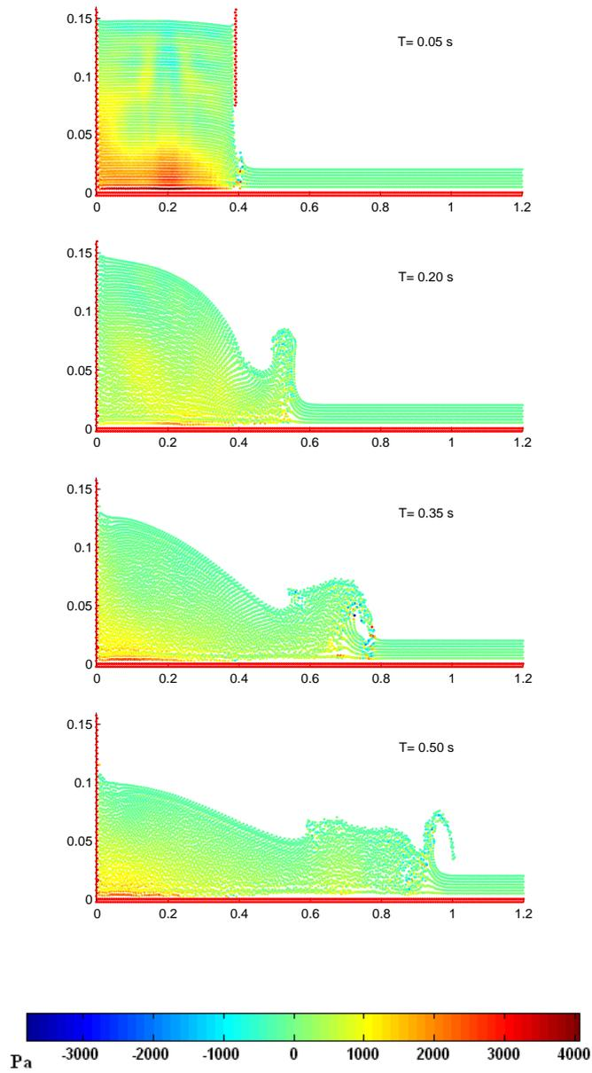
Figure 5.7: Different instants of the dam evolution for the case  $d = 0.018m$ . Pressure field is represented.
