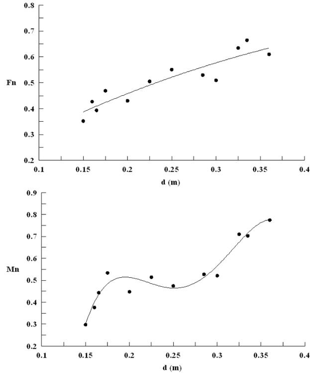
Figure 6.15: Dependence of the normalized force ( $F_n$ ) and normalized moment ( $M_n$ ) on the distance dike-structure for a tall dike ( $H_D = 0.0875m$ ).
