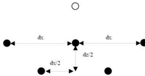
Figure 3.13: Sketch of the interaction between a fluid particle (empty circle) and a set of boundary particles (full circles). The boundary particles are placed in a staggered manner.
