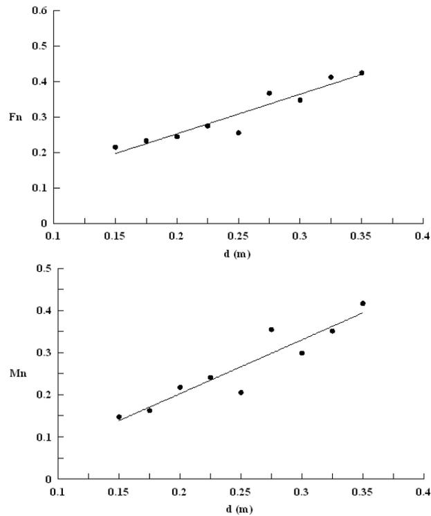
Figure 6.7: Dependence of the normalized force ( $F_n$ ) and normalized moment ( $M_n$ ) on the distance dike-structure for a tall dike ( $H_D = 0.125m$ ).
