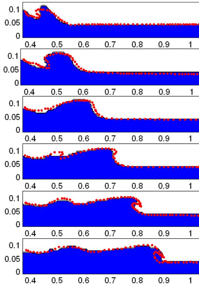
Figure 5.5: Comparison between experimental and numerical profiles of dam-break evolution over a wet bed ( $d = 0.038m$ ). Experimental values are represented by red dots and numerical ones by the blue surface.
