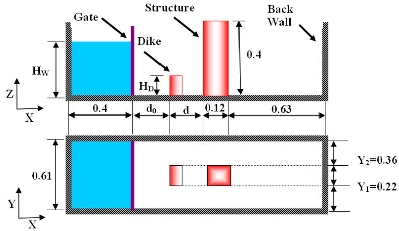
Figure 6.5: Initial configuration of the numerical experiment corresponding to wave mitigation by a dike.
