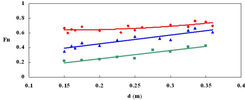
Figure 6.18: Dependence of the normalized force ( $F_n$ ) for different distances dike-structure and different dike heights normalized  $H_D$ ;  $H_D = 0.05m$  (red line);  $H_D = 0.0875m$  (blue line);  $H_D = 0.125m$  (green line).
