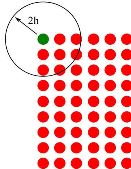
**Particles near edge do not have full support within kernel radius.**
