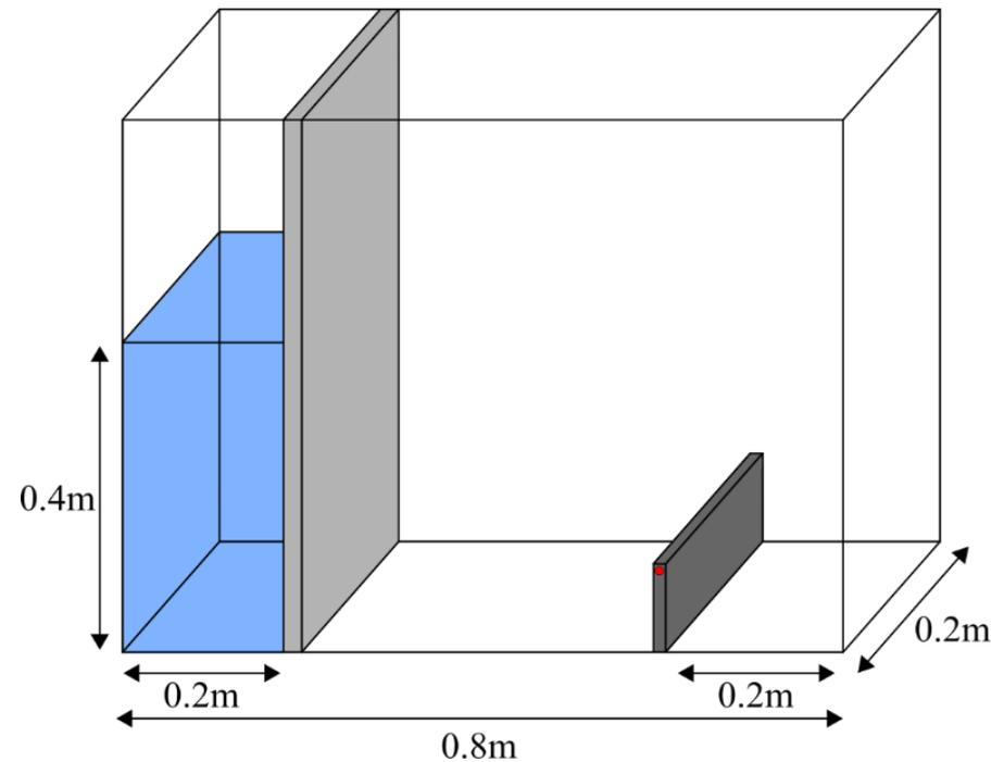
*Schematic of dam break case (Liao et al. 2015).*
