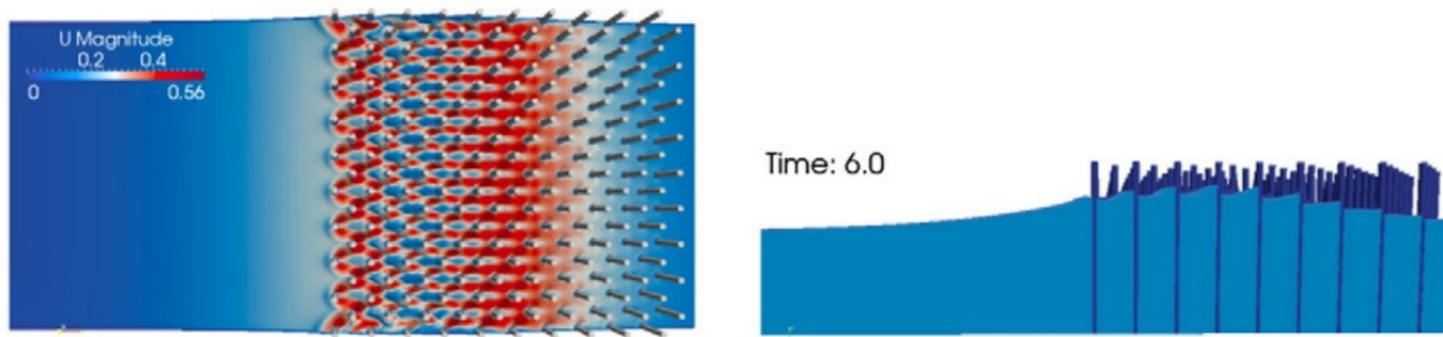
*Flow velocity and surface elevation of wave through array of rigid emergent cylinders (Maza et al. 2015).*
