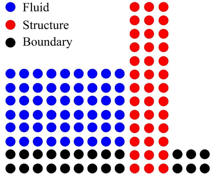
*Particle types used for fluid-structure coupling.*
