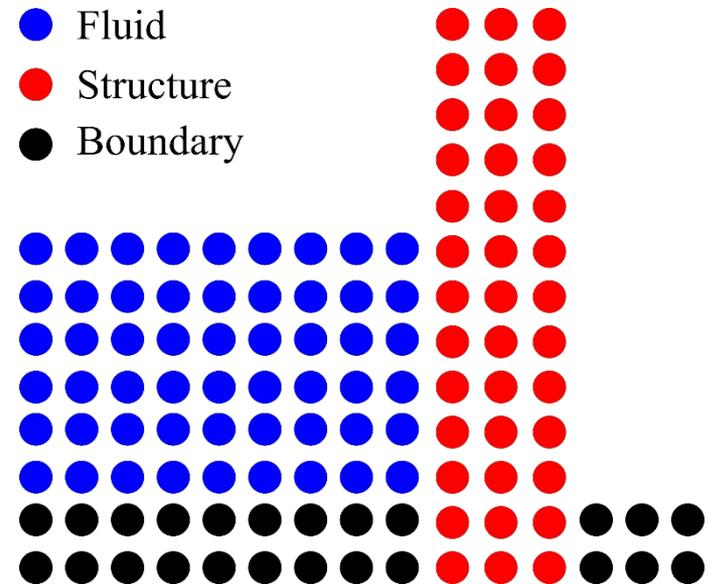
*Particle types used for fluid-structure coupling.*
