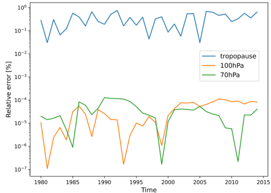
Figure 3.2: Time evolution of the relative error of the decomposition method applied to the ERA5 annual mean data for 1980-2014 at three material lines (70 hPa, 100 hPa, and tropopause).
