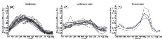
Figure 4. Standardized monthly mean flows, considering all available data from 1949 to 2009 in each region: (a) Atlantic; (b) Mediterranean; and (c) Pyrenean. The blue line represents the mean of the standardized monthly mean flows.
