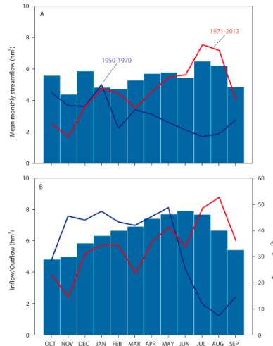
Figure 3. (A) Average river regimes in Boadilla gauge station: blue bars (1950-2013), blue line (1950-1970), and red line (1971-2013). (B) Average monthly values of inflows (blue), outflows (red), and storages (blue bars) in the reservoir of Boadilla between 1971 and 2013.
